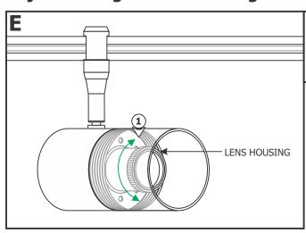
**1:** Rotate the lens housing (inside the fixture body) and set the beam spread to either spot or flood.
