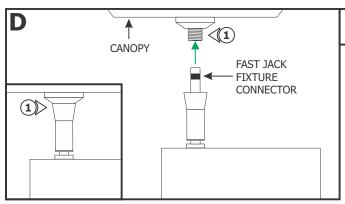
**1:** Use fingers to tighten the Fast Jack fixture connector into the Fast Jack Canopy connector.
