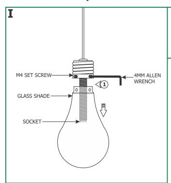
**CAUTION:** To reduce risk of a burn or electrical shock during lamping, disconnect the power to the fixture.
