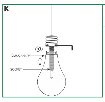
**3:** Align the socket assembly set screws to the glass shade hole. While holding the glass shade in place, secure it by tightening the three M4 set screws with the provided 2mm Allen wrench.
