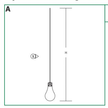
1: Cut the coaxial cable to the desired height (H) with a sharp cutter. The overall fixture height is measured from the bottom of the glass shade to the end of the coaxial cable.
