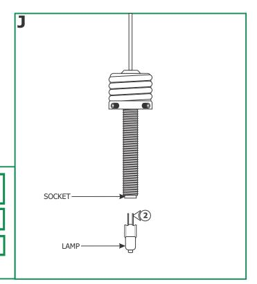
**CAUTION:** To reduce risk of a burn or electrical shock during lamping, disconnect the power to the fixture.
