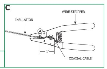
**4:** Use the #12 gauge hole of the AWG wire strippers to strip 1" of the insulation cover from the end so that the bare coaxial cable is exposed.
