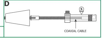
**5:** Feed the coaxial cable into the coaxial fixture connector. The coaxial cable will come to a stop point.
