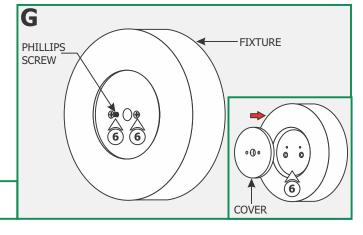
**6:** Replace the cover and secure it to the fixture with the two Phillips screws.
