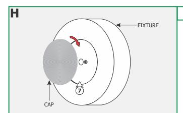
**7:** Tighten the cap onto the fixture to cover the screw holes.
