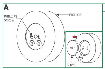
1: Loosen the two Phillips screws to remove the cover.
