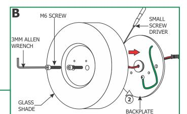
2: Loosen the two M6 screws using the provided 3mm Allen wrench to remove the backplate. Use a small flathead screwdriver to remove the backplate from the glass shade.
