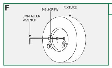
**5:** Place the fixture completely onto the backplate. Replace and tighten the two M6 screws with 3mm Allen wrench.
