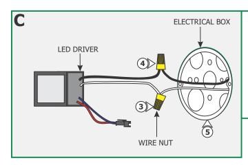
**NOTE:** Turn off power to the junction box before installation.
