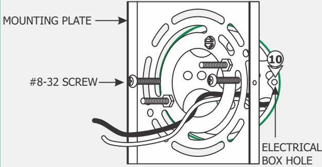
**10:** Mount the mounting plate to the electrical box holes with the provided two #8-32 screws.
