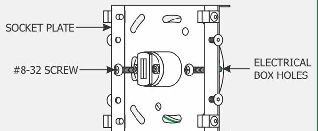
**NOTE:** The mounting plate and backplate can be omitted for indoor locations only if socket plate covers the entire electrical box.
