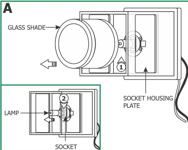
**1:** Carefully unscrew and remove the glass shade from the socket housing plate.
