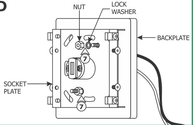
**7:** Remove the two nuts and lock washers to lift the socket plate off of the backplate.
