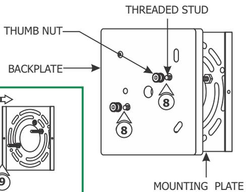
**8:** Remove the two thumb nuts from the backplate threaded studs.
