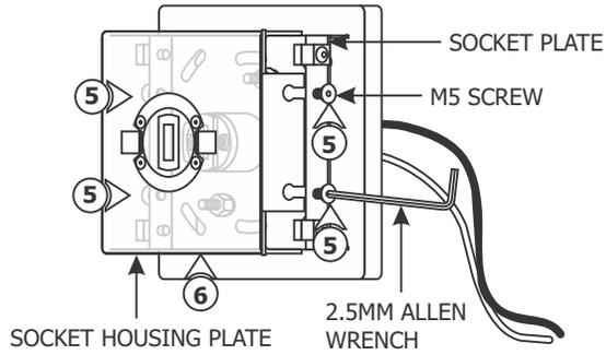
**5:** Loosen the four M5 screws on the sides of the socket plate with the provided 2.5mm Allen wrench (**Do Not Remove**).
