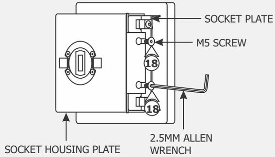
**18:** Push the socket housing plate slots onto the M5 screws and tighten them with the 2.5mm Allen wrench.
