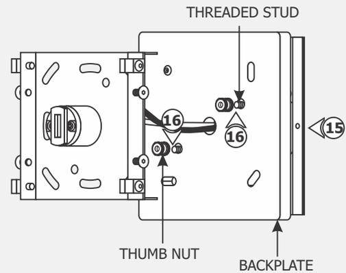
**17:** Replace and tighten the two lock washers and nuts to secure the socket plate onto the backplate.
