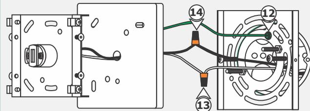
**12:** Connect the backplate ground wire (bare wire) to the mounting plate. Make sure that the mounting plate is grounded in accordance with local electrical codes.
