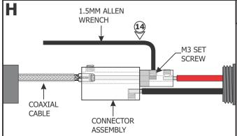
**14:** Use the provided 1.5mm Allen wrench to replace and securely tighten the M3 set screw.
