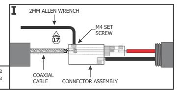
**17:** Use the provided 2mm Allen wrench to securely tighten the M4 set screw until it squeezes the wire ferrule tightly to the coaxial cable.
