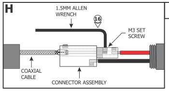
**16:** Use the provided 1.5mm Allen wrench to replace and securely tighten the M3 set screw.
