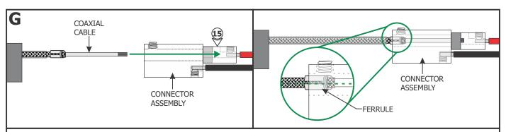
**15:** Insert the coaxial cable into the coaxial connector until the wires of the center conductor are visible through the M3 set screw hole.
