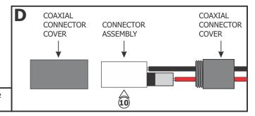
**10:** Unscrew the coaxial connector covers and remove from the connector assembly.
