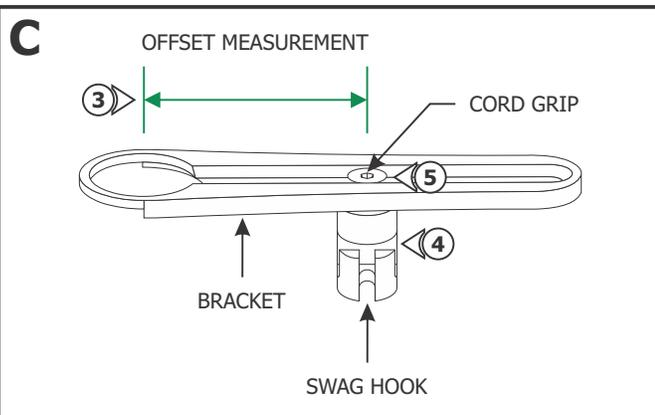
**3:** Determine the offset measurement of the power cords from the center of the M4 screw to the center of the bracket hole.
