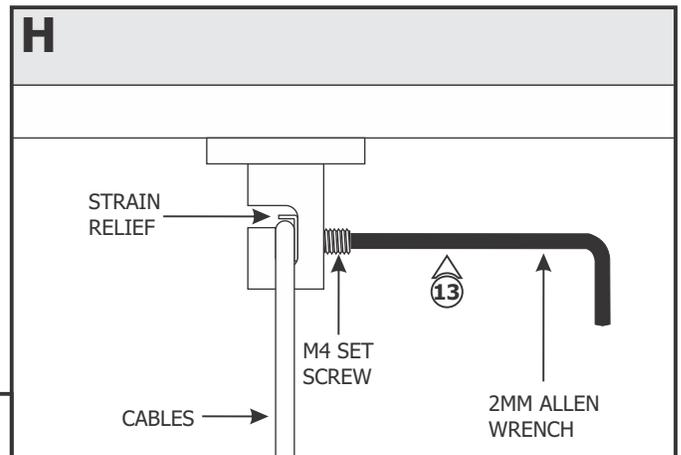
**13:** Tighten the M4 set screw snugly with the 2mm Allen wrench provided to hold the cables in place.
