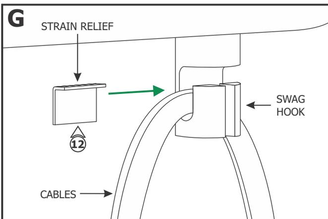
**12:** Insert the strain relief into the swag hook behind the cables.
