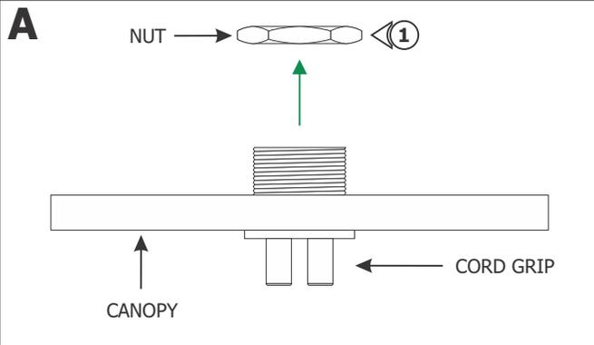
**1:** Remove the nut from the back of the canopy to remove the cord grip.
