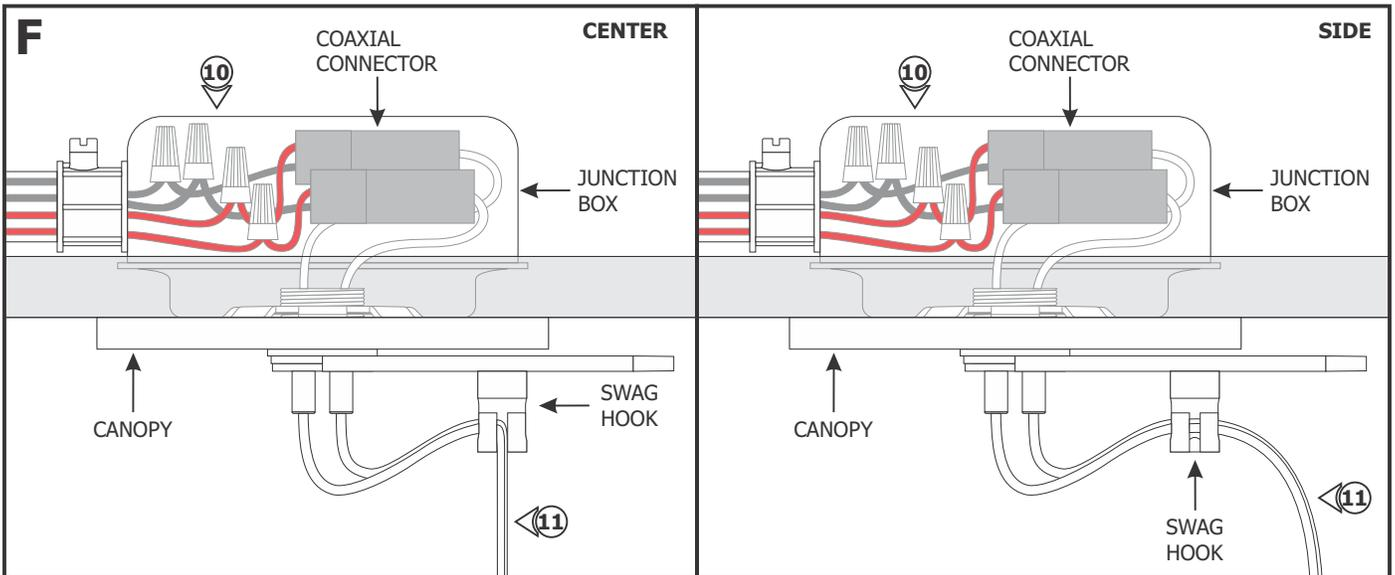
**10:** Refer to the instructions provided with the fixture to install the coaxial connector assembly and canopy.
