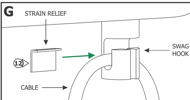
**12:** Insert the strain relief into the swag hook behind the cable.
