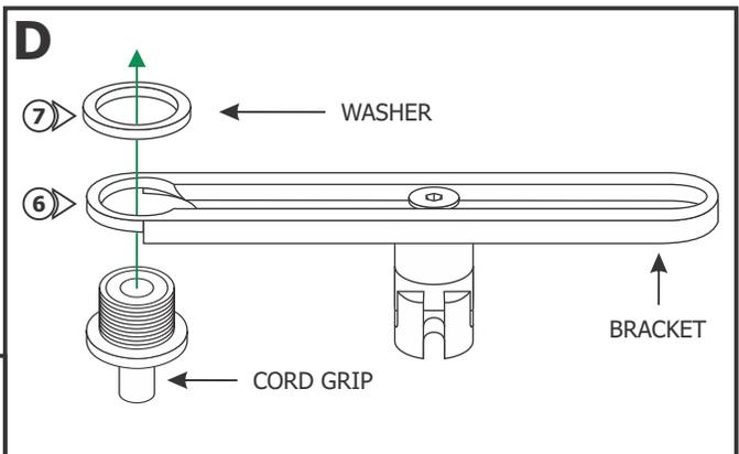
**6:** Insert the cord grip into the bracket hole.
