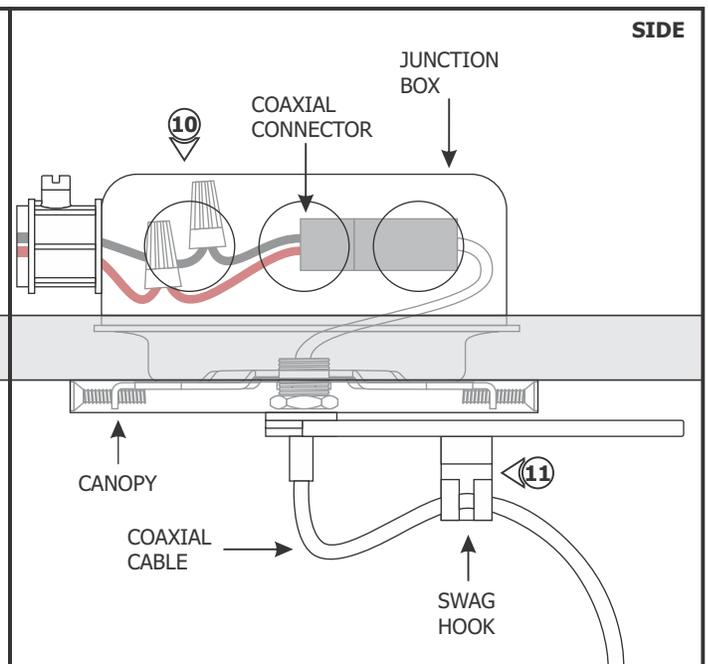
**10:** Refer to the instructions provided with the fixture to install the coaxial connector assembly and canopy.
