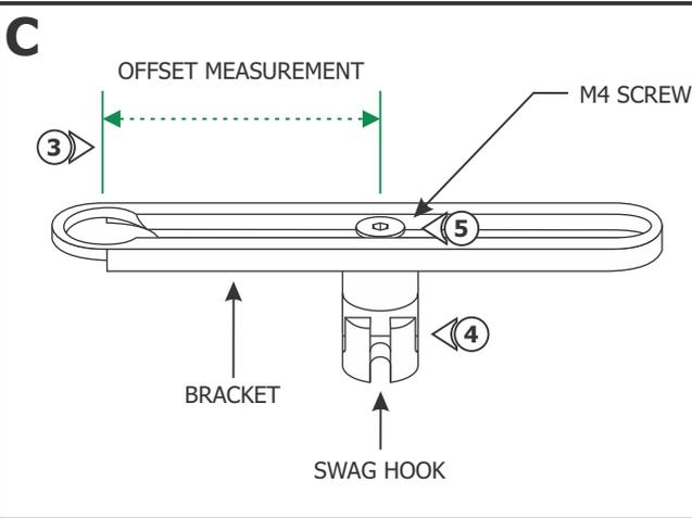
**3:** Determine the offset measurement of the power cord from the center of the M4 screw to center of the bracket hole.
