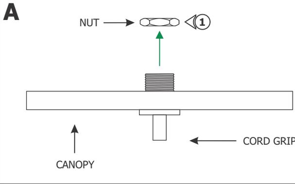
**1:** Remove the nut from the back of the canopy to remove the cord grip.
