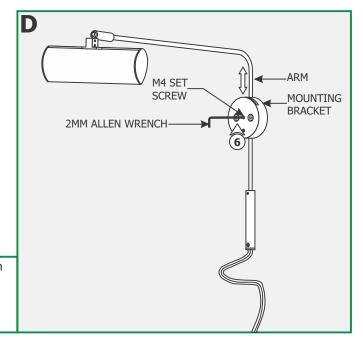
**6:** To adjust the Cody2 height, loosen the two M4 set screws on the mounting bracket with the provided 2mm Allen wrench. Adjust the Cody2 by sliding it up or down. When the desired height is achieved tighten the two M4 set screws with the 2mm Allen wrench.
