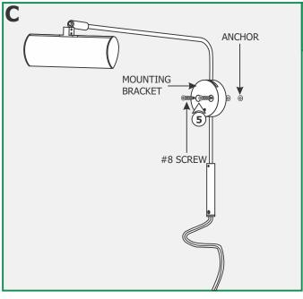
**5:** Line up the mounting bracket holes with the anchors and secure the fixture to the anchors with the two #8 screws provided.
