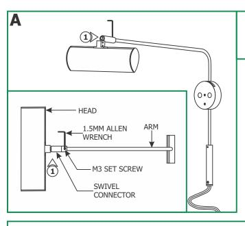
1: Rotate the Cody2's head perpendicular to the arm making sure the arm is completely inserted into the head. Tighten the M3 set screw on the swivel connector with the provided 1.5mm Allen wrench to secure the head in place.
