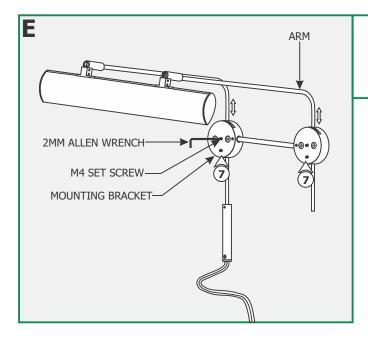
7: To adjust the height, loosen the four M4 set screw on the mounting brackets with the provided 2mm Allen wrench. Adjust the Cody2 to the desired height by sliding it up or down. Tighten the four M4 set screws with the 2mm Allen wrench.
