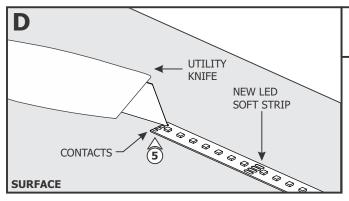
**5:** Place the soft strips on a flat, stable surface. Using a utility knife, carefully scrape the protective coating from the contacts on the ends of each soft strip.
