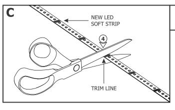
**4:** Determine the amount of new LED soft strip needed. Trim the strip at the marked line above the contacts with a sharp scissor.
