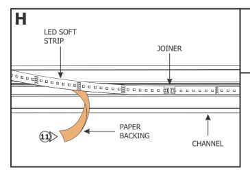
11: Carefully remove the backing from the new LED soft strip, make sure not to remove the tape from the soft strip. Firmly press down the adhesive portion of the soft strip onto the channel while removing the rest of the backing, making sure there are no air bubbles that can cause surface irregularities.
