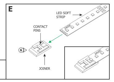
**6:** Insert the old LED soft strip completely into the Snap & Light Straight Joiner. Ensure the soft strip contacts align fully with the contact pins. Push the strip completely into the contact pins.
