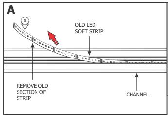
**NOTE:** Avoid bending the soft strip in sharp vertical angles which may damage the LEDs. Soft strips do not bend horizontal. Use proper directional connectors for horizontal turns.
