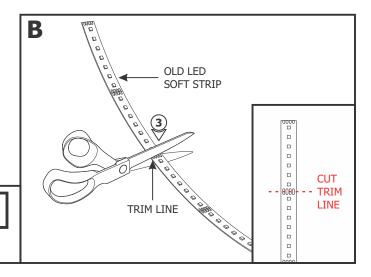
**NOTE:** Do not trim the strip at unmarked sections which may cause that section of the strip to not light up.
