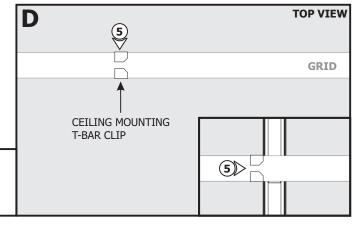
**5:** Place the T-Bar clip onto the grid and squeeze the arms together to secure in place.
