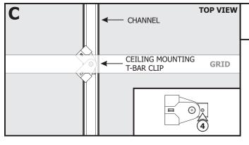
**4:** If aligning the channel perpendicular to the grid, it may be necessary to remove the set screw from the clip to rotate the arms into position.
