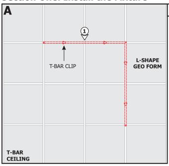
1: Determine the location of the fixture on the T-Bar ceiling.
