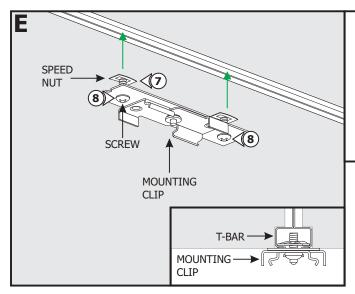
**NOTE:** Omit steps 7 through 11 if using the Ceiling Mounting T-Bar Clips (**TBA** and **TBB**).
