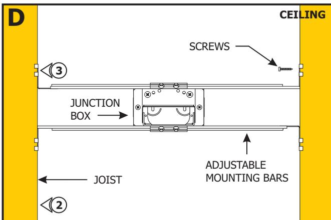
**NOTE:** The adjustable mounting bars mount to joists that are spaced 14.5"-25" apart.
