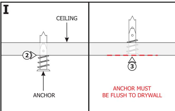
**NOTE:** Steps 2 and 3 are for drywall mounting. Omit these steps if mounting to a wood surface directly.
