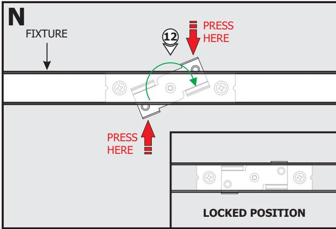
**12:** Twist each locking clip to lock the fixture in place.
