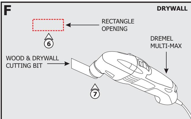
**6:** Mark a rectangle shape on the drywall where the junction box opening will be located depending on the selected position.
