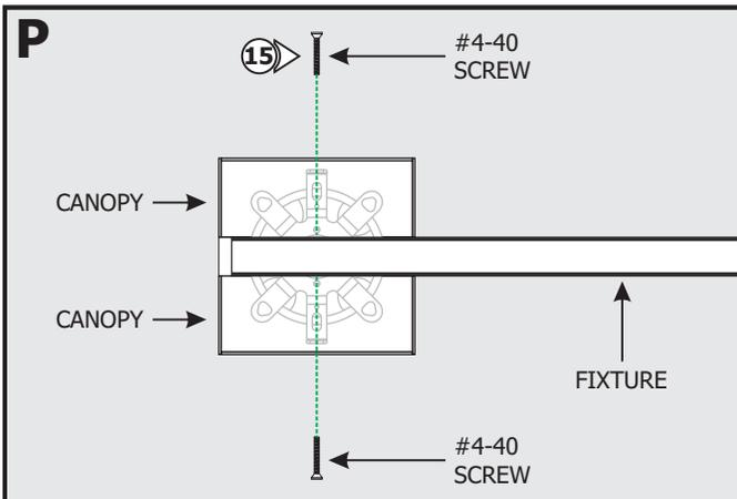
**15:** For 4" Square Split Canopy installations, place each canopy piece against the fixture and align the canopy holes with the crossbar holes. Secure the canopy pieces in place with the two #4-40 screws and 1/16" Allen wrench provided.
