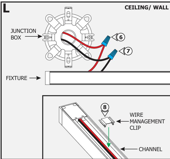
**6:** Connect the low voltage +24VDC power supply wire to the red wire of the fixture using a wire nut.
