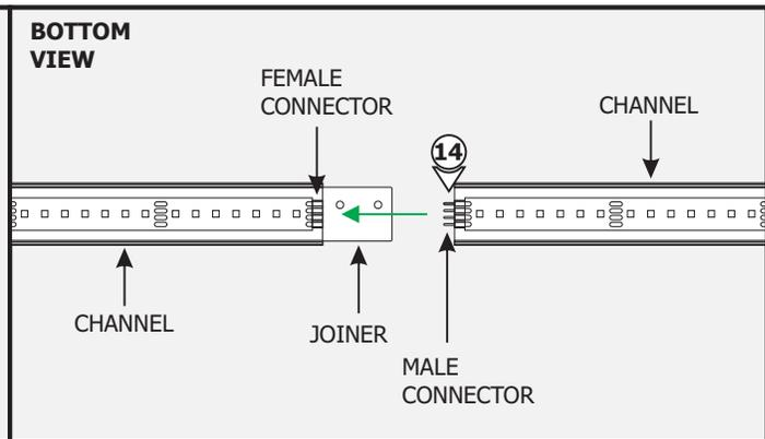
**NOTE:** Omit steps 13 through 16 if the channel is made out of a single piece (120" or less).
