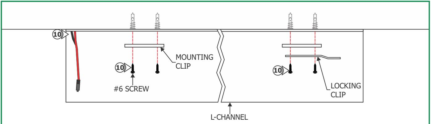
**10:** Insert the power connections into the junction box.
