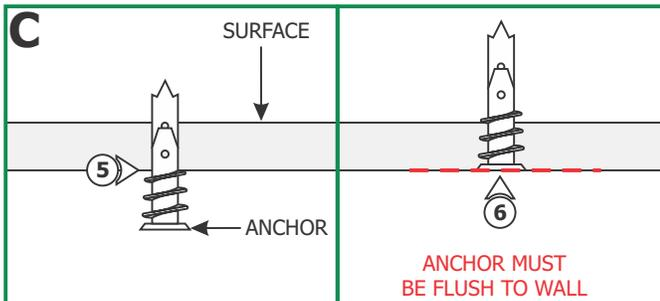
**NOTE:** Steps 5 and 6 are for drywall mounting. Omit these steps if mounting the clips to a wood surface directly.
