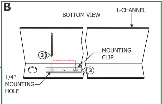
**3:** Mark the location of each mounting and locking clip per the instructions included with the channel.
