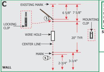
**NOTE:** BV2-IRE is shown for demonstration purposes. **NOTE:** Locking clip must be installed in the opposite direction of the fixture wire. Fixtures greater than 36" are provided with two locking clips. **NOTE:** The junction box could be offset, but needs to be aligned to the center of the channel.
