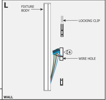
**6:** Refer to wiring diagrams on pages 5 and 6 to connect the wires properly.
