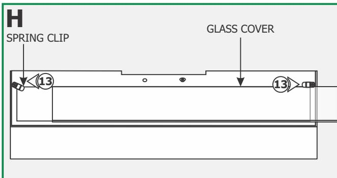
**13:** Loosen the screws on the spring clips (**Do Not Remove**) to insert the glass cover under the clips. Slightly tighten the spring clip screws to secure the glass cover in place.
