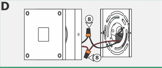
**8:** Connect the red power supply wire to the red fixture wire with a wire nut.
