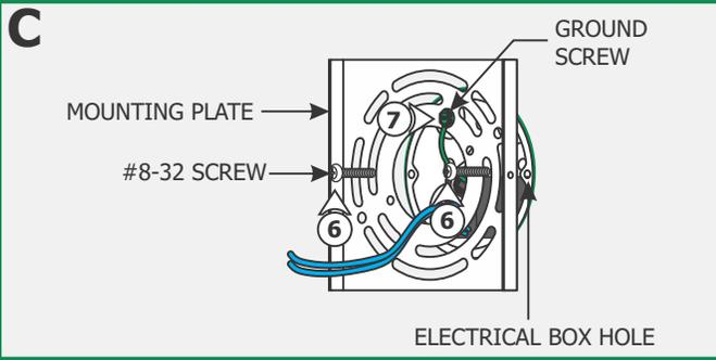
**6:** Line up the mounting plate with the electrical box holes, and secure it in place by tightening the two #8-32 screws provided.
