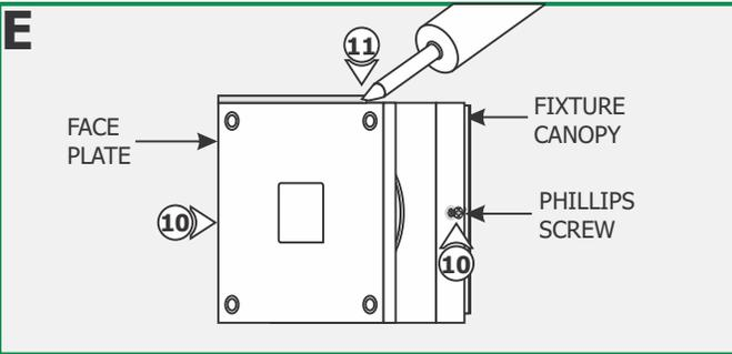
**10:** Place the fixture canopy onto the mounting plate, make sure the gasket is in place and secure it by tightening the two Phillips screws.
