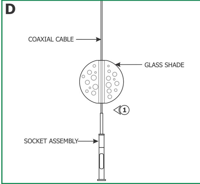
**1:** Feed the coaxial cable through the glass shade, and rest the glass shade over the socket assembly.
